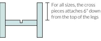
Flip the cross piece for the second assembly so the half laps fit together
